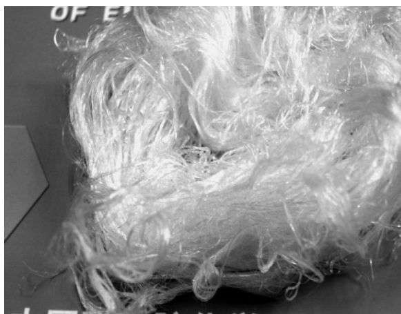
Fig. 2. Cellulose fibers manufactured by dry jet-wet spinning process from AmimCl solution [22].
