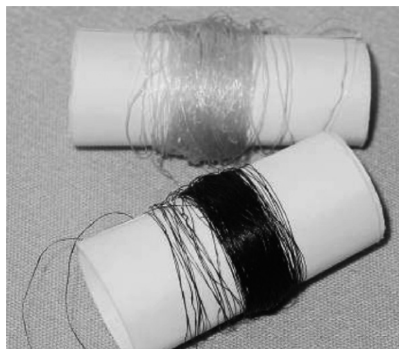
Fig. 5. Photograph of the regenerated cellulose (white) and cellulose/MWCNT composite fibers (black) [26].
